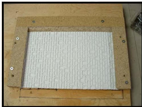
Cut a piece of Precision sheet plastic( with a pattern of your choice) to the exact size of your walls and insert it from the bottom. **Wrong side up** screw the bottom piece in to complete the jig.
