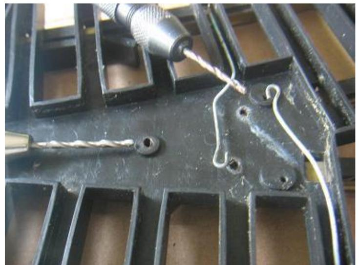
In order to replace the screws you will have to minimally elongate some screw holes in the track bed.
