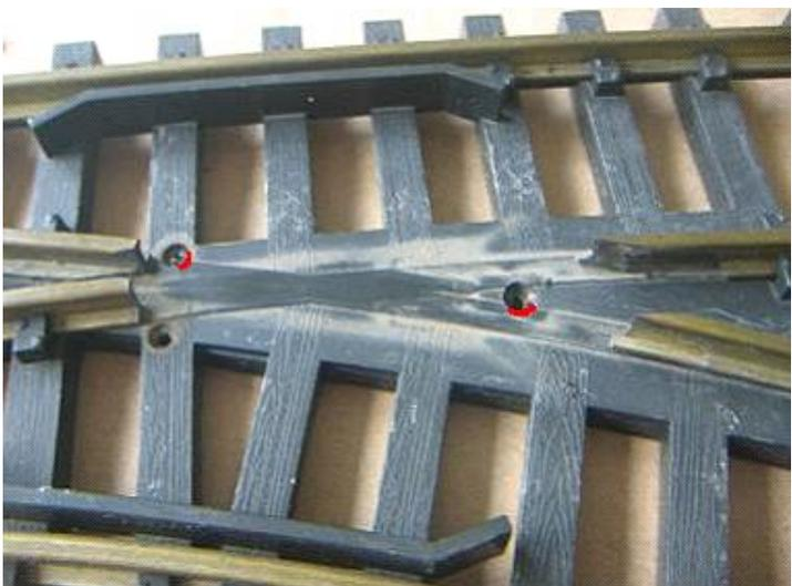
Elongate the indicated dimples very slightly in the direction of the desired rotation. Do not widen the dimples.
