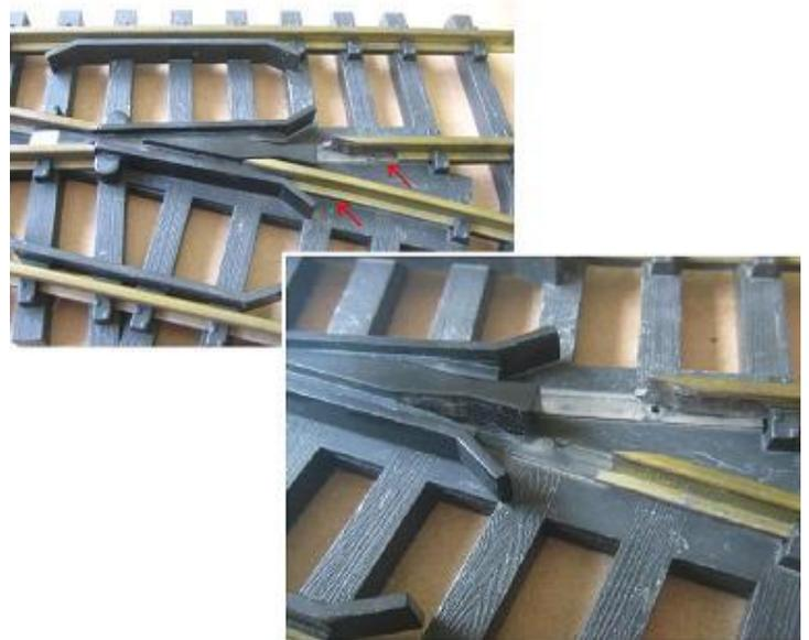
Still keeping close track of where the various screws belong, remove the three screws holding the plastic frog in place. Also locate the screws securing the rails running to the wide end of the frog. They would be just outside this picture, to the right....
